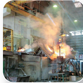
Melting in an electric furnace
