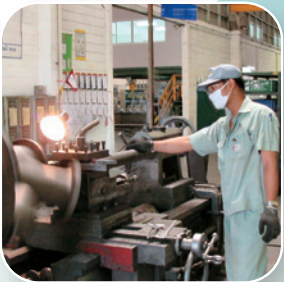
Machining large workpieces on a lathe
